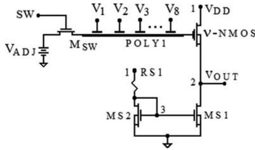
Figure 26. Configuration of the quasi-FGMOS v-NMOS neuron.
