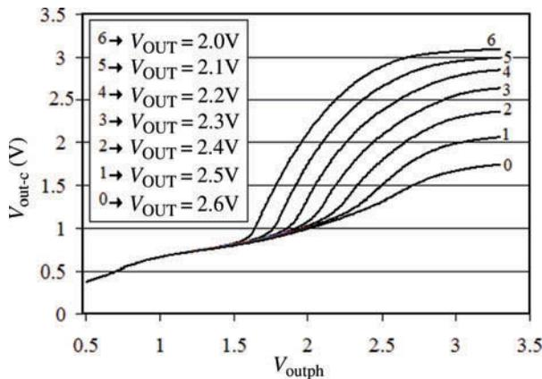
Figure 22. Parametric transfer function for the comparator.
