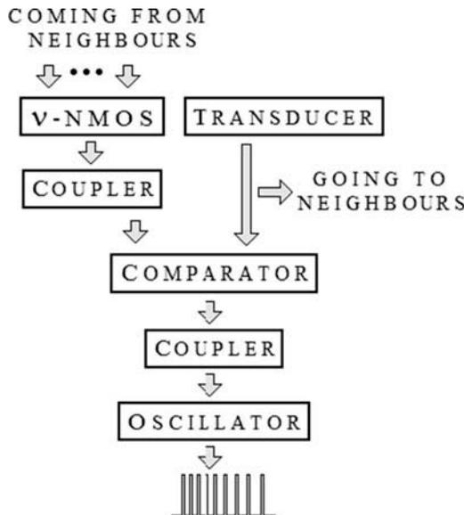
Figure 13. Architecture of each pixel.
