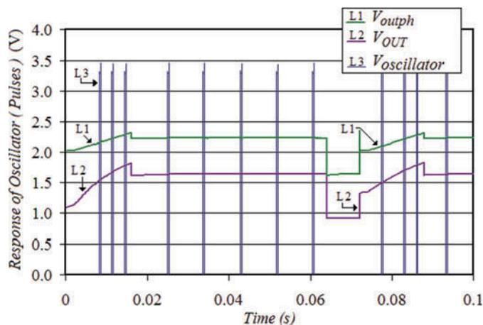
Figure 23. Pulses delivered by the oscillator.
