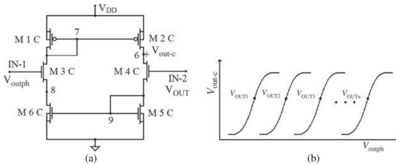
Figure 16. Comparator: (a) schematic; (b) ideal response.
