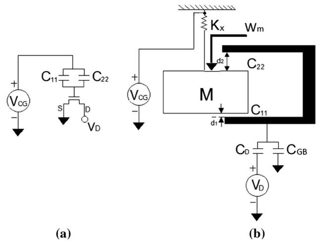
Fig. 5 a Electrical diagram for the inertial sensor; b electromechanical diagram for inertial sensor
