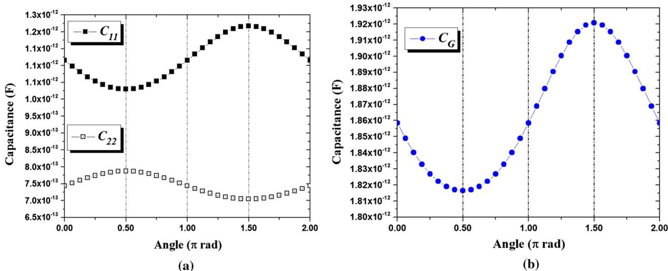
Fig. 6 a Behavior of the components  $C_{11}$  and  $C_{22}$  obtained from (7) and (8), respectively; b total behavior of  $C_G$  obtained from (9)
