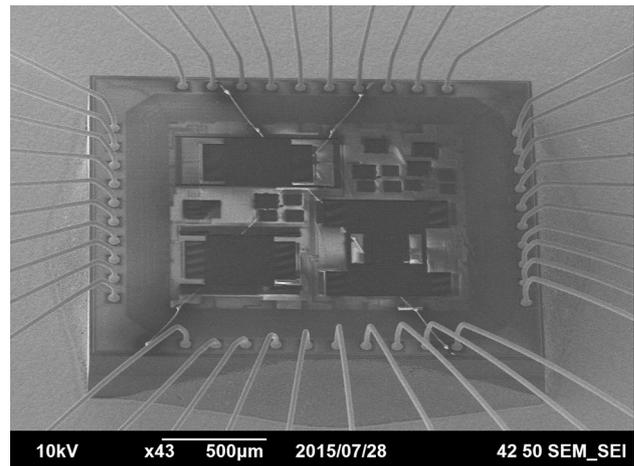
Fig. 11 Packaged chip after MEMS post-processing
