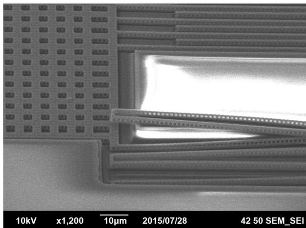
**Fig. 13** Mass supported by the spring, with the SEM holding plate rotated 70°
