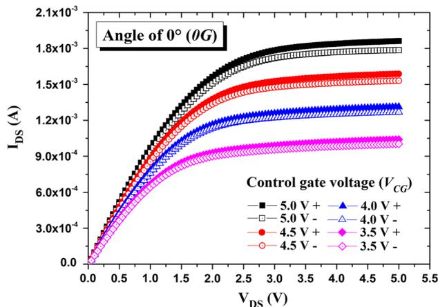
**Fig. 15** FGMOS output curves, horizontal position ( $0^\circ$ , 0G), where  $V_{CG}$  is the control gate voltage
