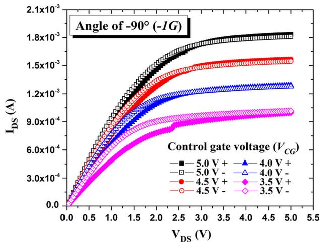
**Fig. 17** FG MOS output curves, - 90° tilt, where  $V_{CG}$  is the control gate voltage
