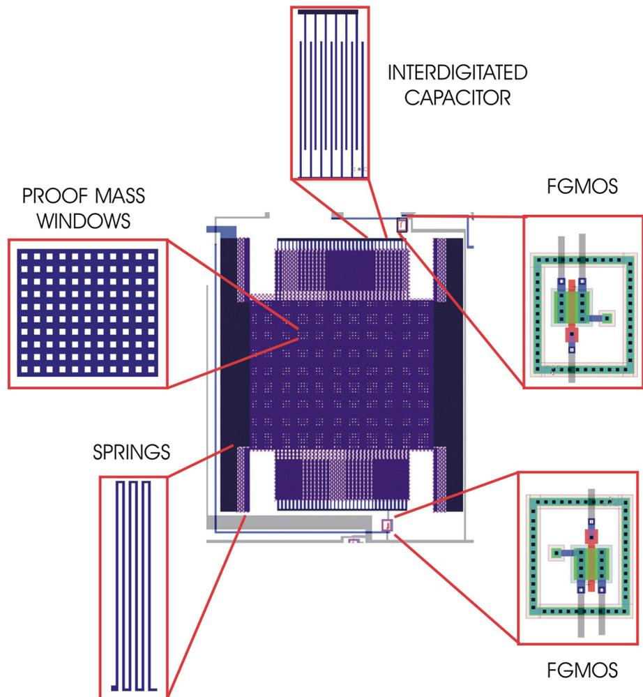
system, whereas the other plate is formed by the opposing fingers in the corresponding fixed electrode, this is, the gate of the transistor. An interdigitated comb array of capacitors is built with the side walls of both pairs of comb electrodes, and since the whole electromechanical structure is intended to be micromachined to allow movement, the dielectric will be air. Figure 8 illustrates the configuration, showing in a simplified way the mass, the springs and the comb capacitor.
