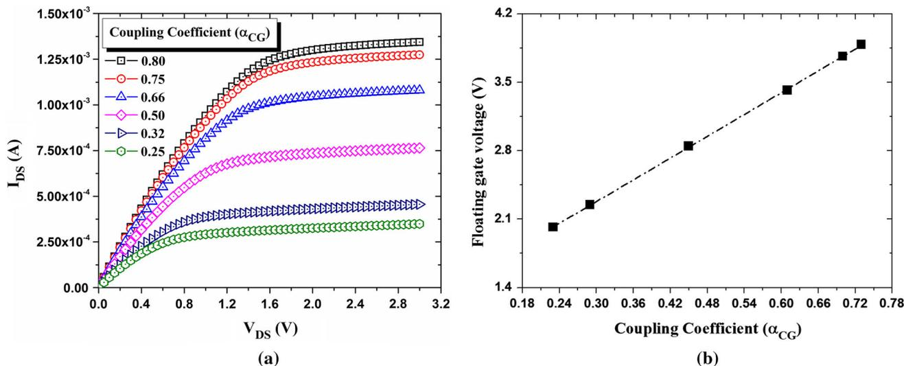
Fig. 7 a I–V output plot for a FGMOS with different coupling coefficients; b  $V_{FG}$  vs  $\alpha_{CG}$
