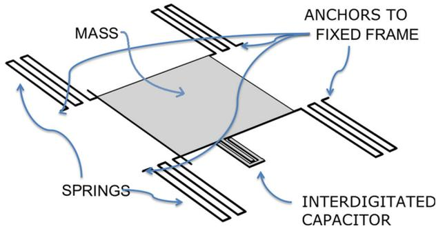
Fig. 8 Electromechanical configuration of the inertial structure
