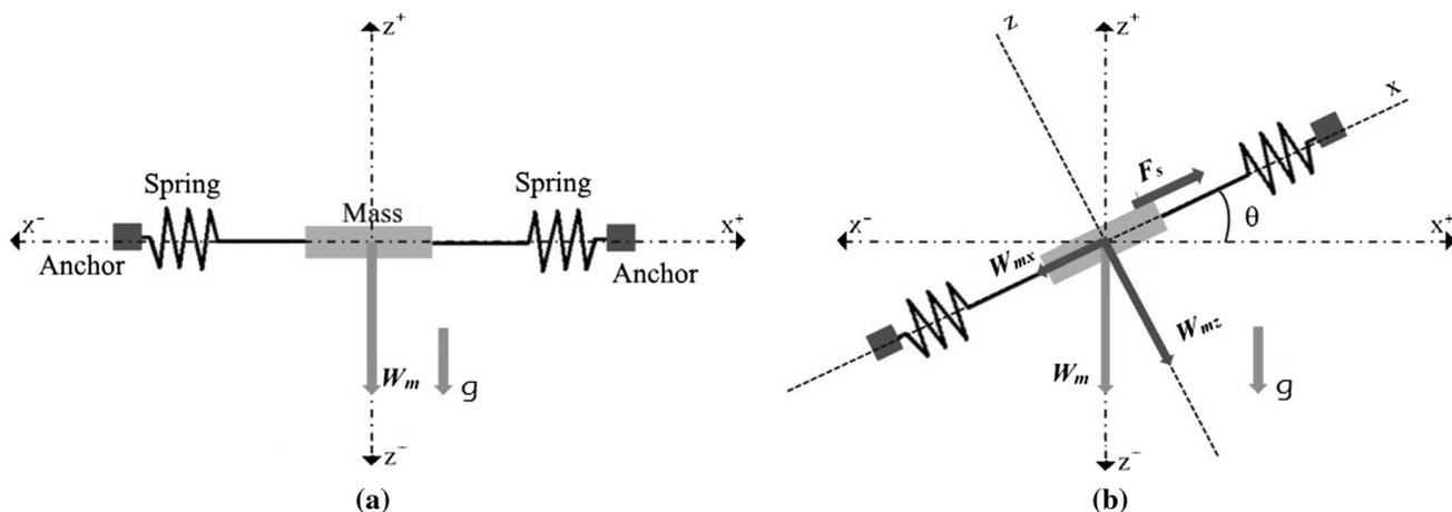
**Fig. 4** **a** Mechanical structure at  $0^\circ$  tilt; **b** tilted structure, showing components of applied force
