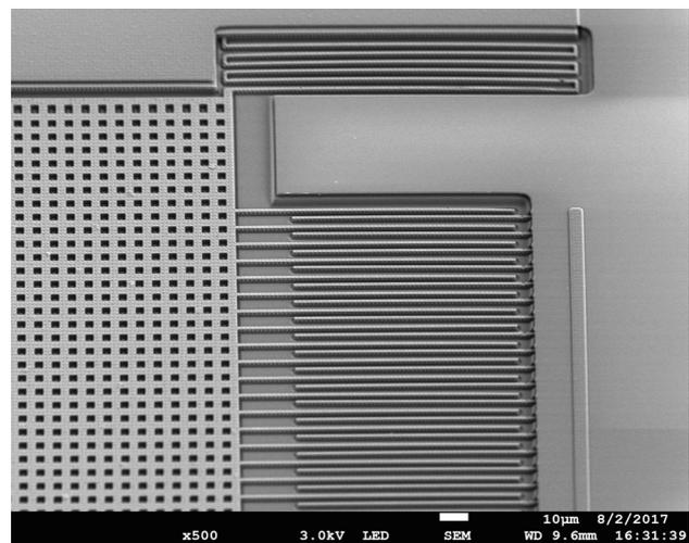
Fig. 12 The inertial mass (left) and the frame (right), forming the control gate capacitor ( $C_G$ )
