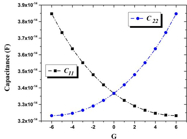
Fig. 10 Behavior of the control gate capacitance for both FGMOS included in the proposed design
