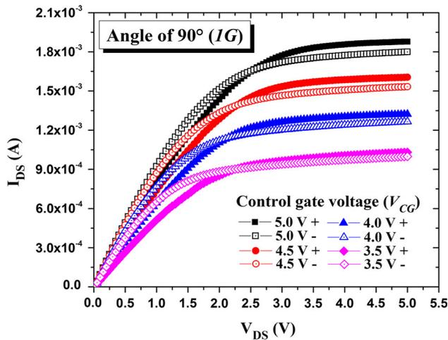
**Fig. 16** FG MOS output curves, 90° tilt (1G), where  $V_{CG}$  is the control gate voltage
